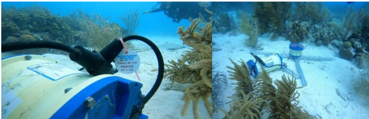
Figure 4: Example of a moored ADCP measurement set-up
