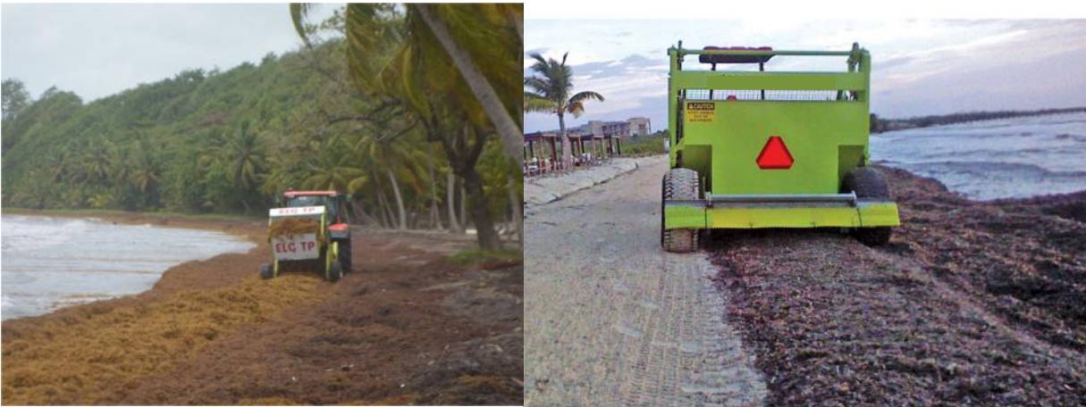
Mechanised beach rakes in action in Guadeloupe (left) and picking up Sargassum, in Mexico (right).
