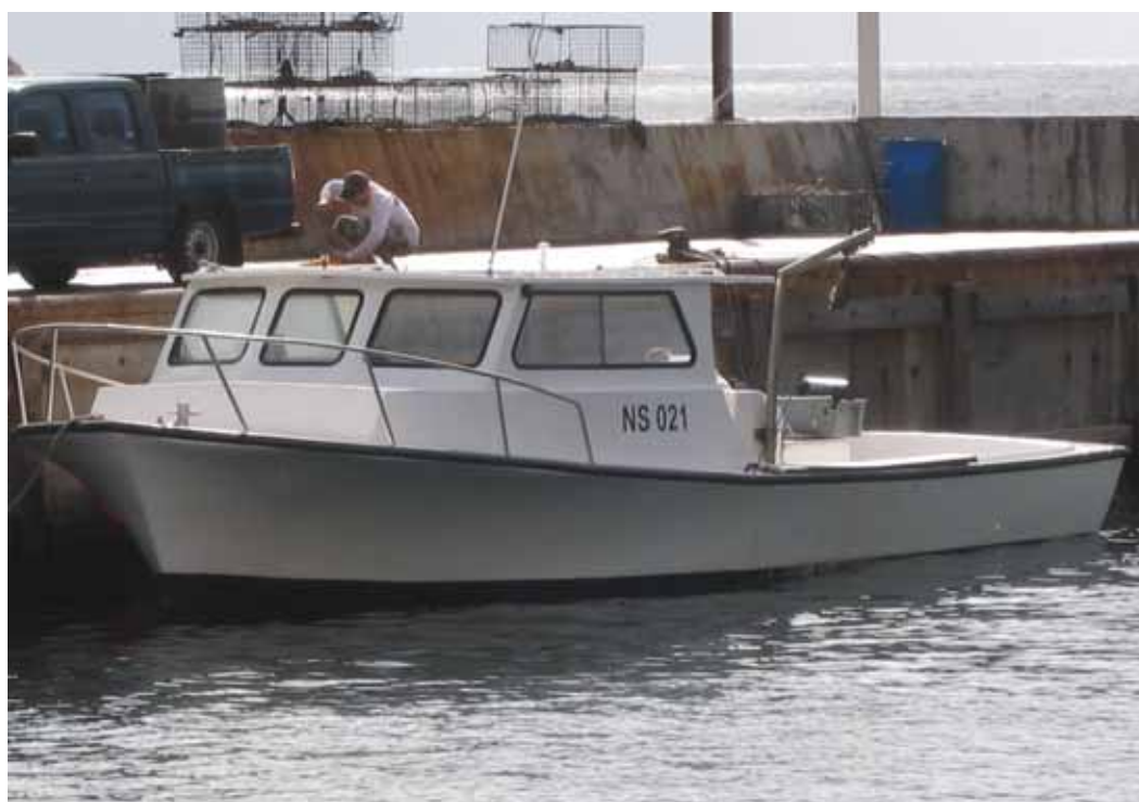
Figure 2. A typical commercial fishing vessel used for trap fishing on Saba Bank. Note the davit and hydraulic wench mounted to port side behind the wheelhouse.
