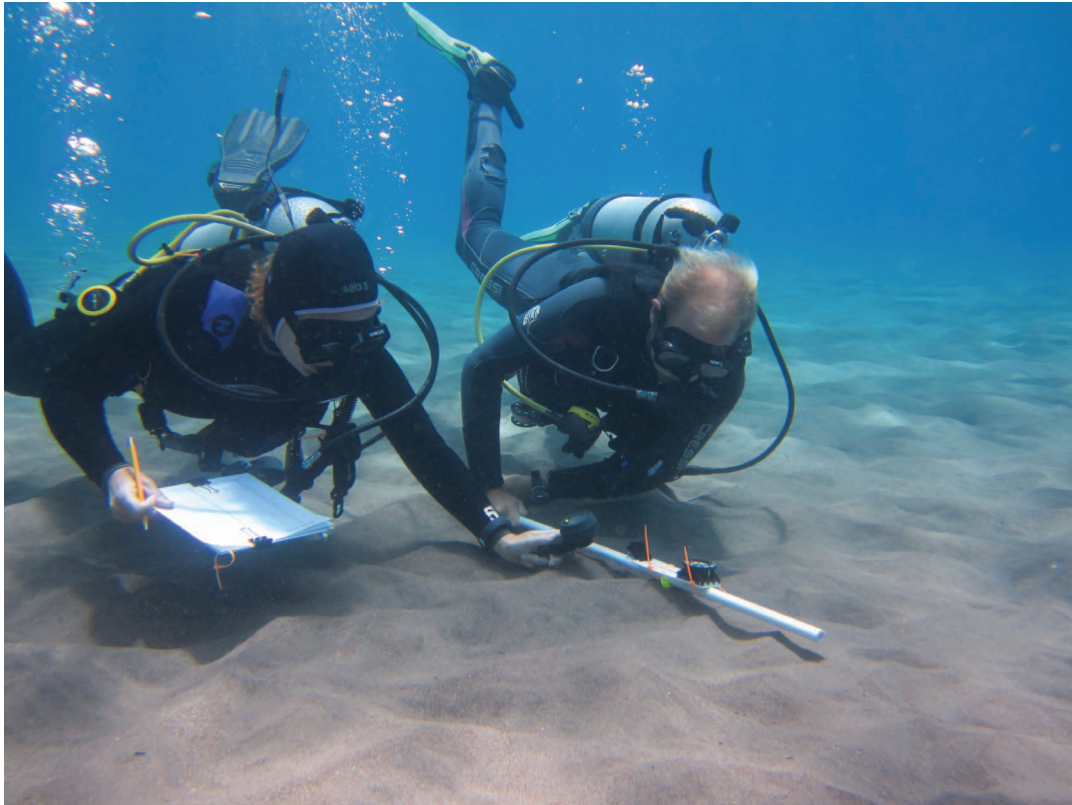
Figure 2. Photo of diver depth-gauge profiling (DDGP) technique. Person on right orients and moves the meter stick. Person on left reads and records depth at each meter. A video of the process can be seen on YouTube at http://youtu.be/0yMtwU5xGuQ . (Color for this figure is available in the online version of this paper.)
