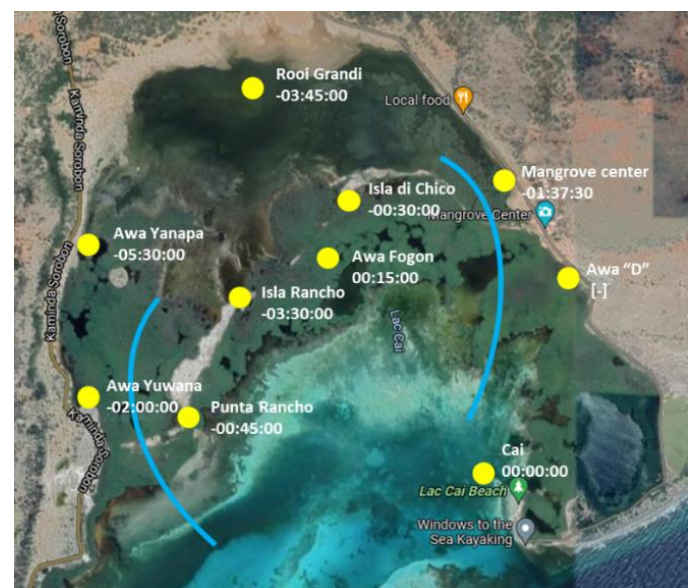
Figure 6: Timing of the high water (averaged) in relation to measurement station Cai including probable paths of the tide (blue lines)
