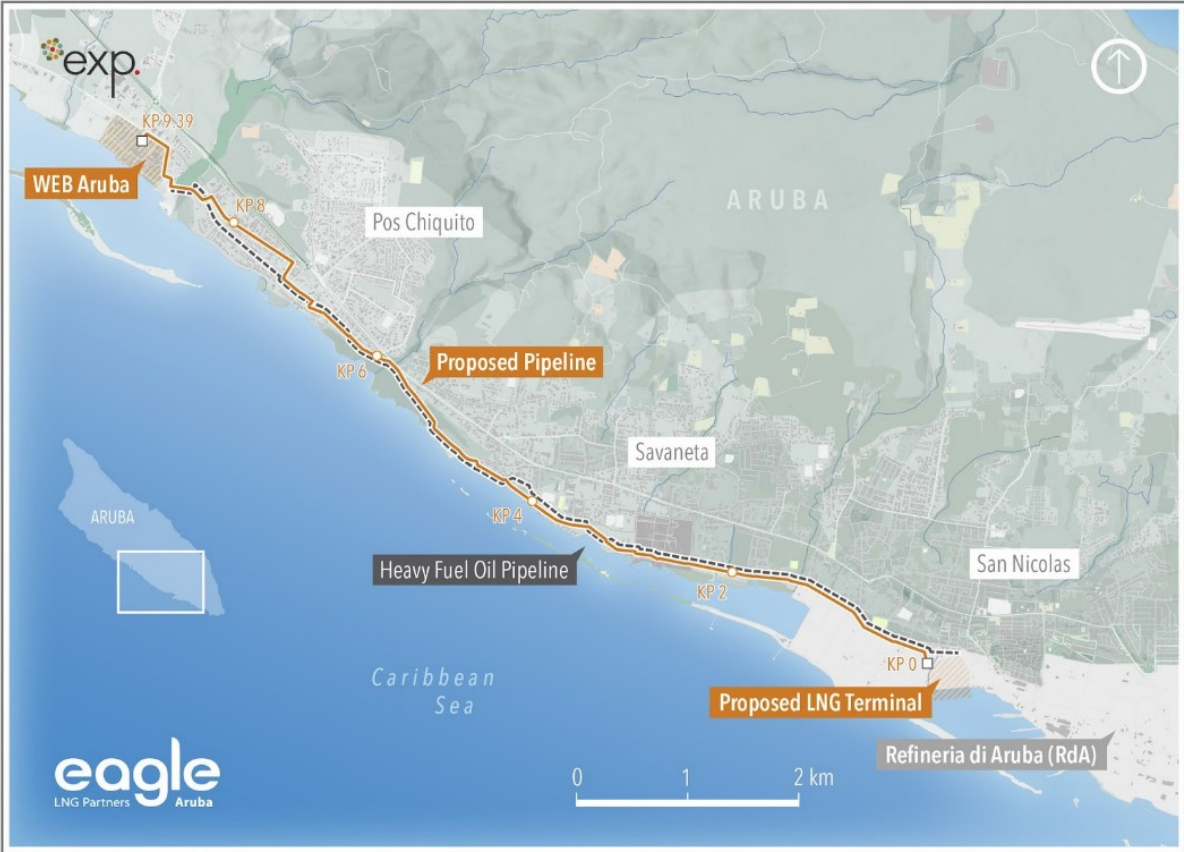
Figure 1: Pipeline route (Lacle, 2022)
