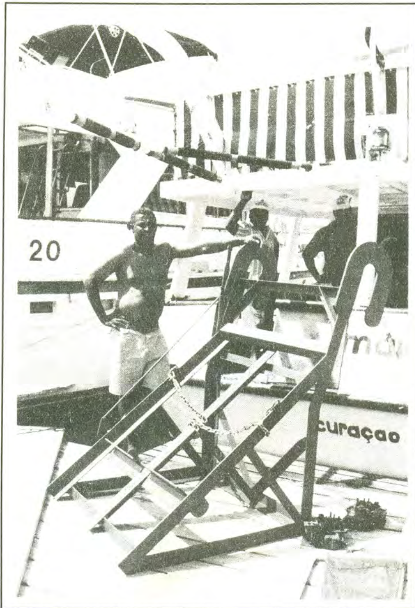
Figure 17 Anchor launching ramp with small chain to secure anchor block. Stern of launching vessel, M/V Mermaid , to which this ramp is fastened can be seen in the background.
