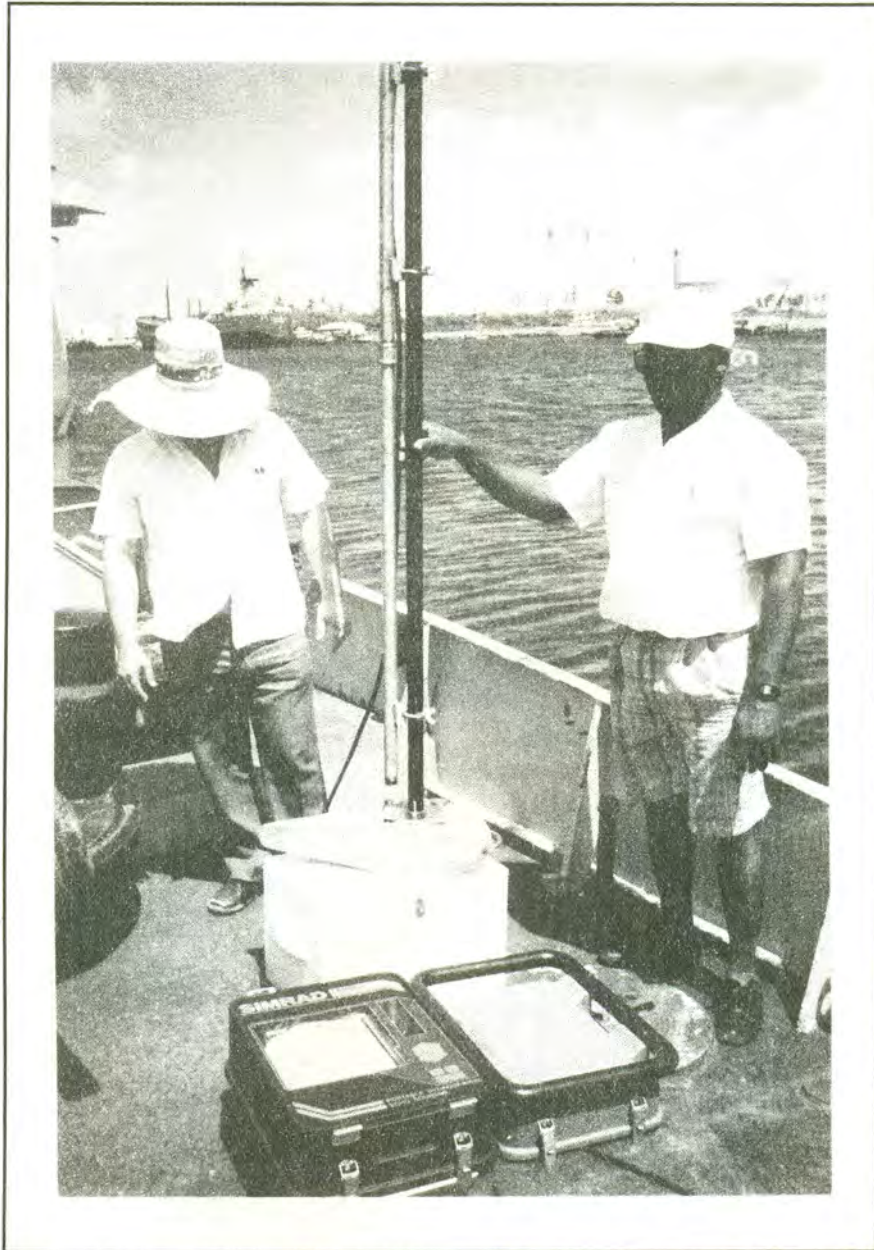
Figure 12 Simrad EA 300 P portable hydrographic echo-sounder. Transducer mounted in a wooden fish (the fish must be turned 180°, to reduce strain on black pole to which transducer is screwed).
