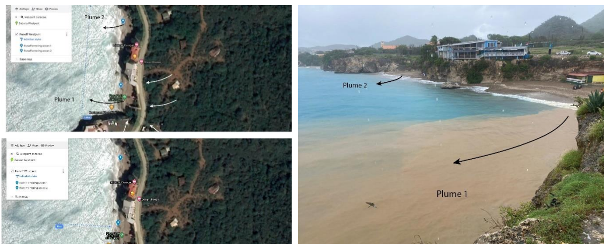
Figure 55. Runoff stream direction and flow as witnessed at Westpunt. Curaçao. Dashed arrows are added to illustrate where witnessed streams are expected to originate from as based on height map Curaçao. Estimation of length plume 1 after rainfall had stopped is roughly 80 meters ( Google Maps Locations ). Runoff streams entering the ocean at Westpunt, Right: Curaçao in November, 2020 during heavy rainfall. Picture taken from Restaurant Playa Forti. Plume 2 formed as rain continued.
