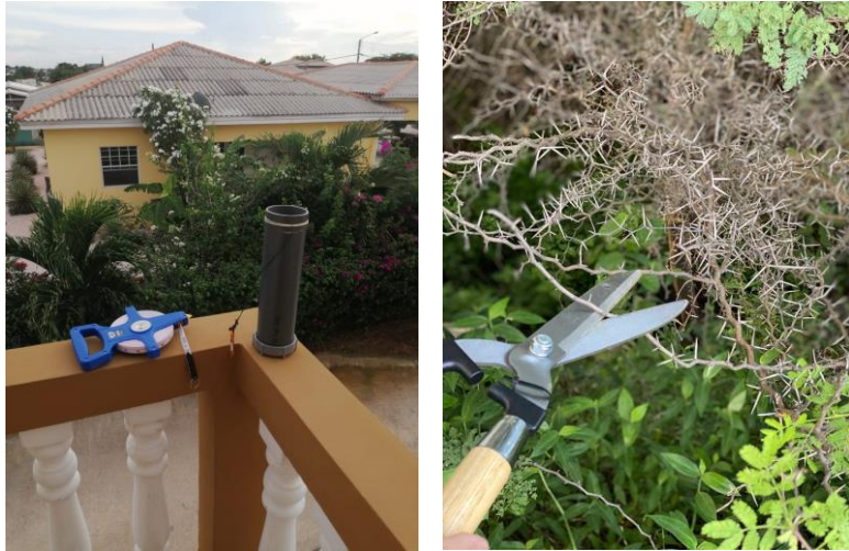
Figure 8. Field work material. Left: groundwater sampling device. Right: hedge cutters to get through bushes.
