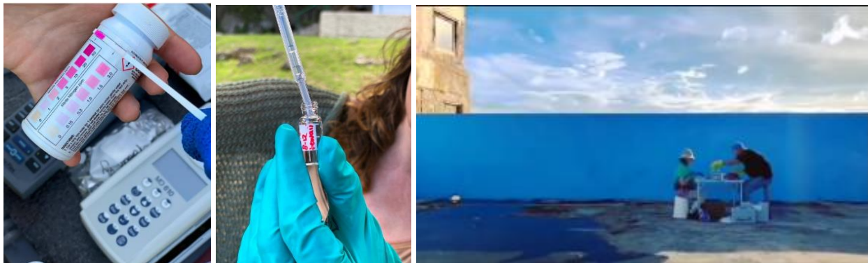
Figure 9. Fieldwork material & portable field lab. Left: Nitrate strips and Lovibond MD610. Middle: Filling the 2 mL vial for stable isotope analysis in the Netherlands. Right: making sure the parameters are measured in time.
