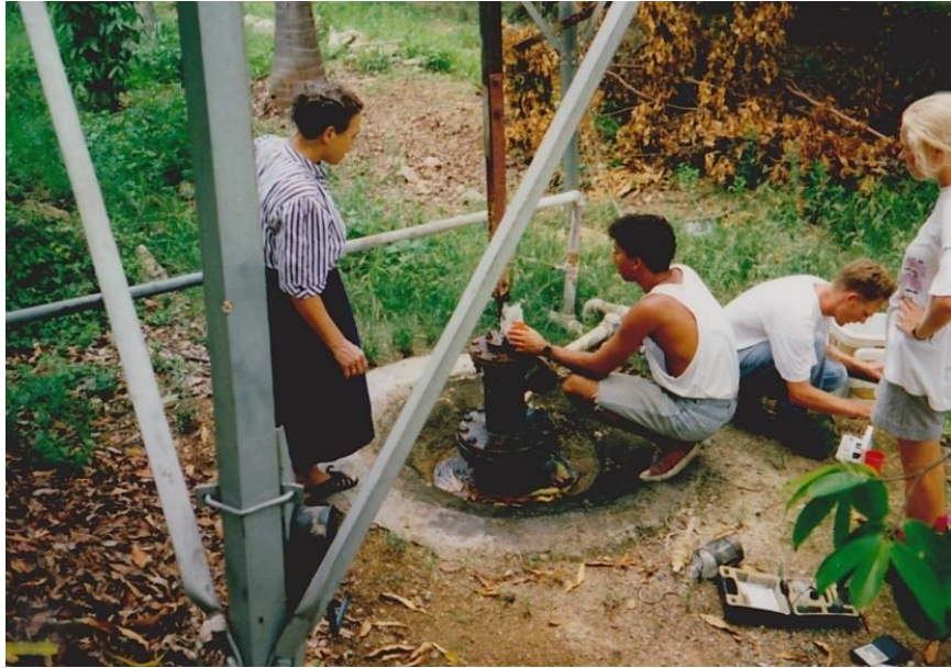
Figure 16. Sampling in 1992. In 1992 a heavy bottle was used to retrieve the groundwater.
