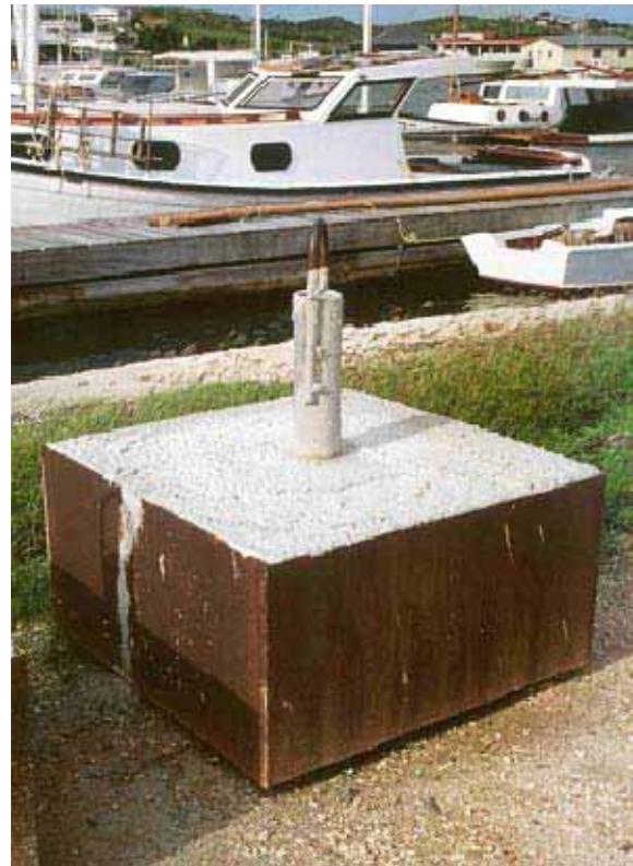
1 500 kg anchor The weight of the anchor has been increased from 1 260 kg to approx. 1 500 kg The underwater weight of the anchor is approx. 1 000 kg
