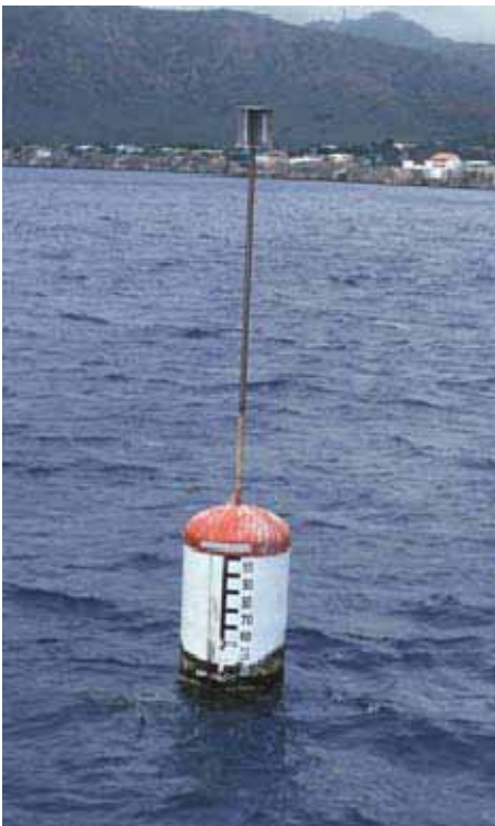
MKII-GRP8 Weak current 430 m mooring depth Considerable reserve buoyancy remaining
